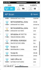
view allows filtering by any field for efficient troubleshooting, while the graphical view provides a clear visualization of cochannel and adjacent channel interferers.
