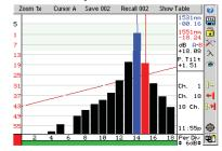
The FTE-8000-CWDM graph display can be configured to optimize the test view. The user can zoom in on specific channels, mark the display area in which channels meet power criteria, limit the number of overall channels viewed and as shown here display power tilt indicator.
