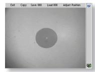
The FTE-8000-CWDM will accommodate the TTI CI1100 Video Probe allowing the user to visually check connectors for cleanliness and damage prior to testing. This helps eliminate costly repairs to the fiber optic connects on the FTE-8000 and results in more accurate tests.
