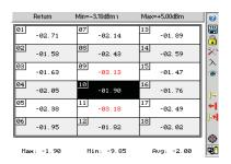
In the table view, the FTE-8000 displays failed channels in red and when a channel is highlighted, statistical information is displayed including the minimum, maximum and average power levels.
