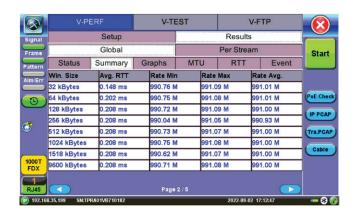
V-PERF is a hardware-based benchmarking test for network performance at different TCP window sizes, to verify stateful TCP/UDP throughput at full line rate, understand KPIs that may be causing network congestion and speed degradation, optimize window sizes, and assure the link meets the required quality of service (QoS).
