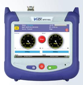
The MTX150x Lite is an optimized Quality of Experience (QoE) test solution (Layer 4+ applications) for multi-Gigabit services from 10 Mbps to 10 Gbps, on copper and fiber interfaces. This rugged and ultra-portable hand-held test set helps field technicians install, verify, maintain and troubleshoot high-speed Residential and Business services, Internet Access and other packet-based services up to 10 Gbps. Native support for 2.5G/5G/10GBASE-T reduces cost of ownership.
