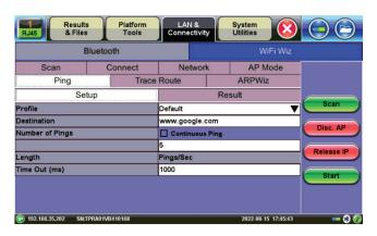
IP: IPv4 (Static, DHCP) and IPv6 (Static, Auto) and PPPoE VLAN support, Ping, Trace Route check
