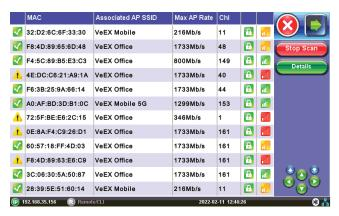
The Air Expert Client scan function monitors all WiFi channels to detect WiFi clients with the SSID they are associated to, as well as non-associated clients (clients not connected to an AP). Network administrators can ensure that the devices are authorized on the network by checking against their MAC address and manufacturer information as well as monitor the client's activity.
