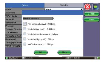
Service calls and end user frustration can often be traced to the common complaint of a "slow network." The Air Expert's V-Perf test can help to unequivocally prove the WiFi network's capacity. With configurable data transmission rate and Pass/Fail threshold, technicians can quickly establish whether the achieved upload and download rates meet SLA requirements and readiness for high bandwidth traffic like audio and video streaming.
