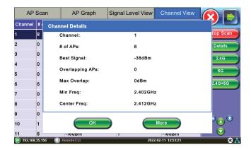
Detailed channel measurements can be sorted by any field including utilization %, number of APs, number of co-channel APs and strongest signal. This information is crucial as technicians need to identify if performance issues are linked to high channel utilization and must quickly decide if reconfiguring the AP to a new channel is advisable.
