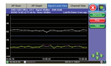
With user configurable thresholds, it is easy to pinpoint where the Signal or Noise levels fall below acceptable quality and ensure site readiness. With a set of pre-configured and configurable location labels, add location information to your measurements to create a full record of the facility walk through.
