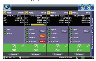
Up to two concurrent sync sessions can be used simultaneously verify physical, link and packet timing performance. A separate test port can also be used to generate Ethernet traffic (Throughput test) to stress the network, link and/or Boundary Clocks (T-BC). Run simultaneous Master and Slave emulations on Module 1, with or without SyncE physical layer synchronization, for localized T-BC configuration verification and troubleshooting.
