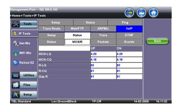
**VoIP Call Expert** – Emulates an IP phone and can place and receive calls using SIP or H.323 protocols. Comprehensive Codec support and call destination options verify voice encoding and translation provisioning. Real-time evaluation of subjective voice quality (MOS and R-factor) is made possible using the patented Telchemy® test method.
