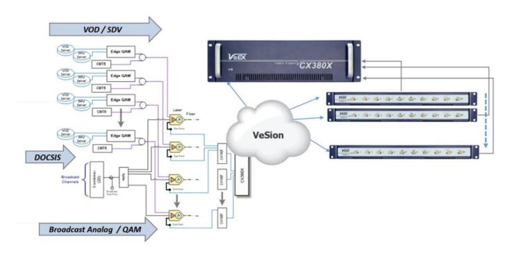
Note: Each CX380X can support multiple CX180F probes to support Forward Path monitoring applications.
